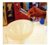
**3.** Glycerol is added using a measuring cylinder. As glycerol is very viscous and sticks to the wall of the measuring cylinder, it should be rinsed with some sterile distilled or cold boiled water and then emptied into the bottle/tank.
