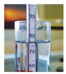
**3.** The alcoholmeter shown in this information pamphlet is for use with ethanol; if used to control an isopropanol solution, a 75% solution will show 77% (± 1%) on the scale at 25°C.
