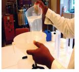
1. The alcohol for the formula to be used is poured into the large bottle or tank up to the graduated mark.
