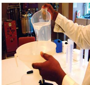
1. The alcohol for the formula to be used is poured into the large bottle or tank up to the graduated mark.
