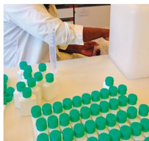
7. Immediately divide up the solution into its final containers (e.g. 500 or 100 ml plastic bottles), and place the bottles in quarantine for 72 hours before use. This allows time for any spores present in the alcohol or the new/re-used bottles to be destroyed.
