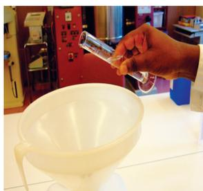
3. Glycerol is added using a measuring cylinder. As glycerol is very viscous and sticks to the wall of the measuring cylinder, it should be rinsed with some sterile distilled or cold boiled water and then emptied into the bottle/tank.
