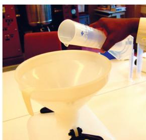
2. Hydrogen peroxide is added using the measuring cylinder.
