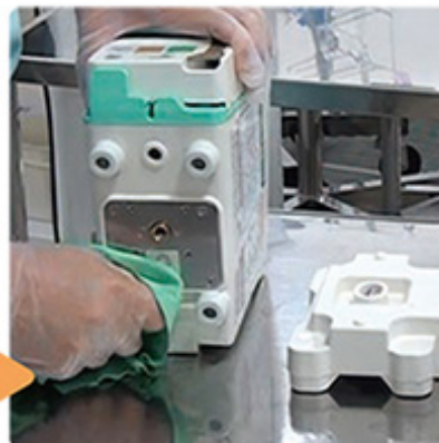
Remove the pole clamp and wipe inside the device and the unit itself.
